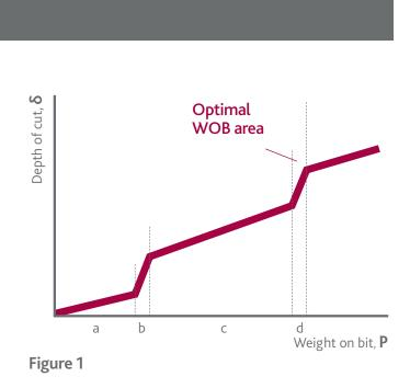
When only a minor impact energy is applied there is only minor fragmentation made by the insert on the rock surface (residual deformation). This results in the rock cracking around the insert contour.
