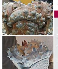
A CONE TOOTH IS BROKEN (LOWER SECTION REMAINS IN PLACE).
