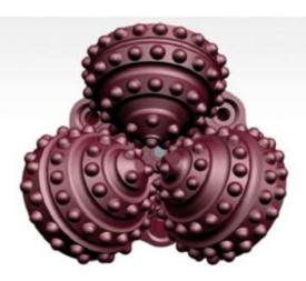
**Pilot bits** are utilized for pilot hole drilling during raise boring operations.
